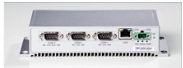
Thycon power system monitor (back)
