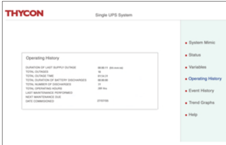
UPS power system monitor - operating history
