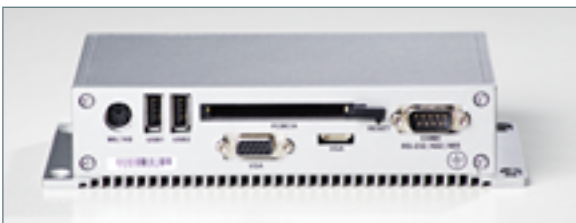
Thycon power system monitor (front)
