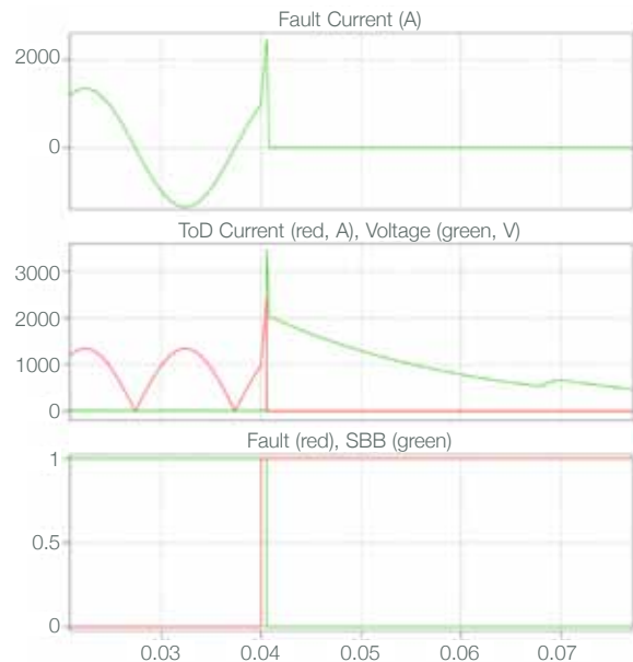
Fig. 5 – Fault current (top trace), ToD current and voltage (centre traces) and fault and turn-off signals (lower traces). Circuit has prospective symmetric fault current of 9.5kARMS
