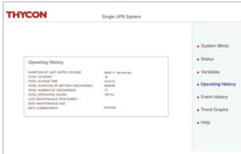
UPS power system monitor - operating history
