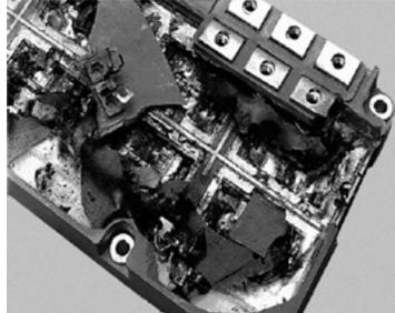
Fig. 2. Failed IGBT module
