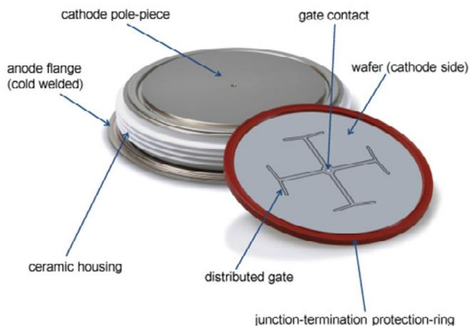
Fig. 4. Wafer and complete press-pack thyristor
