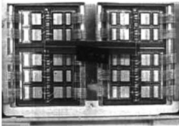
Fig. 1. Wired IGBT substrate prior to encapsulation
